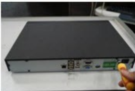
Figure 15-1 Removing the NVR Cover
