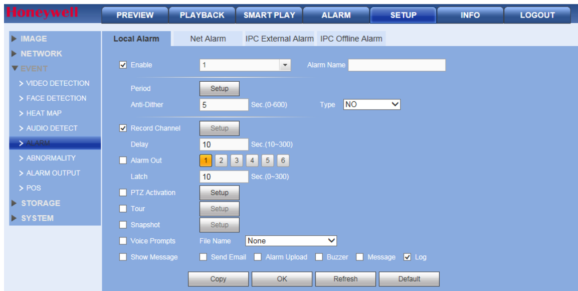
Figure 12-71 WEB - Local Alarm Configuration Interface
