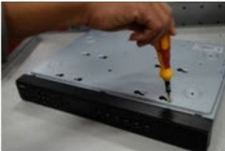
Figure 15-4 Securing the HDD to the NVR Housing
