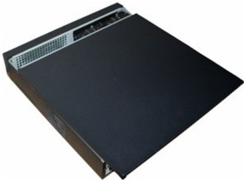
Figure 15-12 Replacing the NVR Cover
