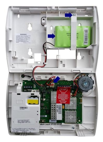
3. Re Install new battery, Screw in battery holder and close system.
